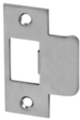
STK Strike (Supplied Standard) Dimension: Conforms to ANSI 115.2 for 1 3/8" doors (2 3/4" x 1 1/8" with curved lip and box) To order with lockset: Designate "STK"
