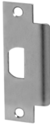
S3 Strike (ANSI Strike) Dimension: Conforms to ANSI 115.2 for 1 3/4" doors (4 7/8" x 1 1/8" with curved lip) To order with lockset: Designate "S3"
